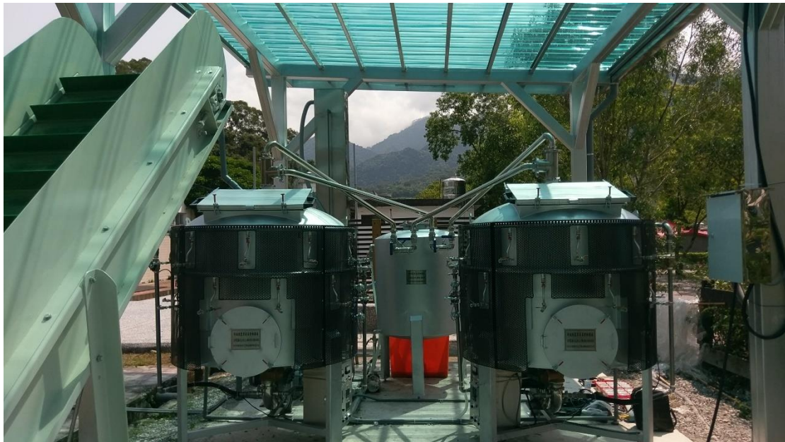
Figure 2. Rapid energy-saving carbonization furnace system.
